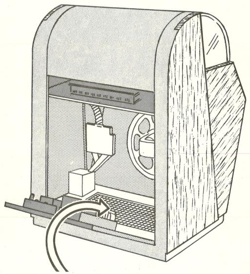
MAKE SURE THE SCREEN IN THE BOTTOM OF THE SELECT-O-MATIC IS CLEAR AND THERE IS AT LEAST A 2-INCH SPACE BETWEEN THE BACK OF THE CABINET AND THE WALL
